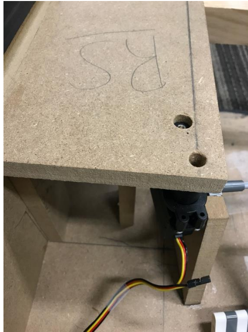
Figure 10: right servo motor and its supports
